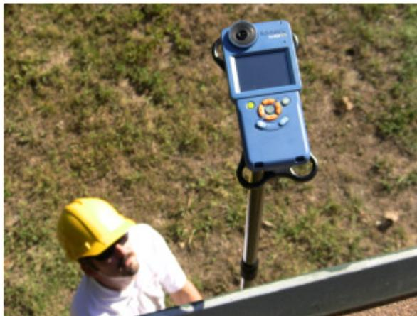
Figure 7. SunEye Extension Kit enables measurements up to 18 feet above ground level.
