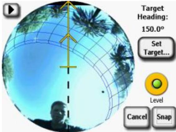
Figure 6. SunEye measurements can be aligned with a known reference when metal interferes with the compass.
