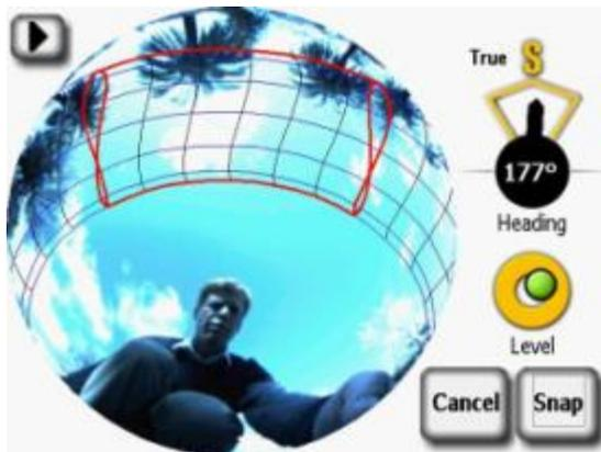
Figure 5.. Identify shade-free areas using SunEye window.
